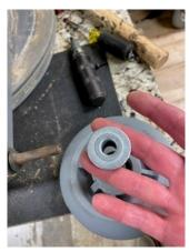
5. Put washer on screw then apply supplied Loctite 242. Thread screw in axle and tighten.
