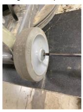
3. Remove the Wheel and nylon spacer. Keep the flat washer for use later.
