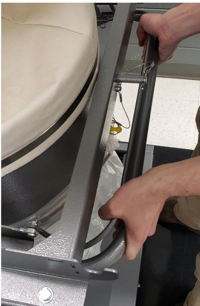
3. While squeezing the bail, lift up on the handle. This will raise the blower assembly of the machine. Once the blower assembly of the machine is approximately lifted half way, release the bail. Continue lifting the handle until you have reached maximum extension. Release the handle and the blower assembly should remain locked on both sides in the extended position. If both sides are not locked, pick up on handle until both locks are secured.
