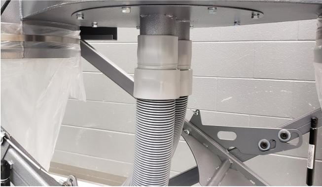
9. Secure the two dust collection hoses to the Gym Vac and the rider. Secure in a manner that prevents the hoses from dragging on the floor and obstructing the operator's access to the rider or view. The bungee cords supplied with the Gym Vac can be used to secure the hoses.
