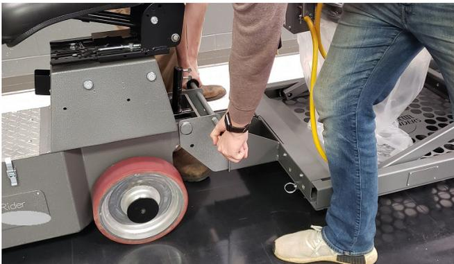
**Note:** In the event the receiver on the rider is not square with the rider, the Gym Vac may connect to the rider at an angle. This will result in the Gym Vac extending further to the left or right of the rider at an angle. This can be corrected with the following:
