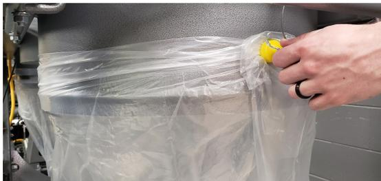
6. Bring the bag clamp up around the bag and clamp on the exhaust outlet. Be sure to clamp above the rib and below the magnet. Repeat process for both bags.
