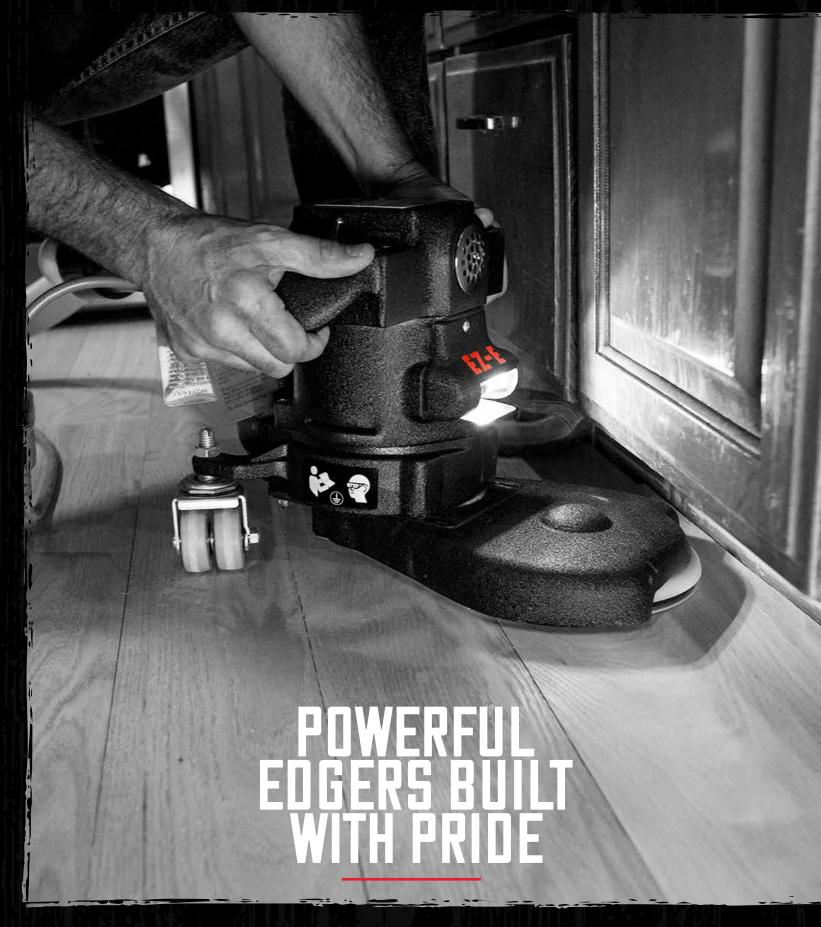
The EZ-E Extension Edger is the perfect tool for tackling the most difficult edging challenges, including toe-kicks and radiators. Available in 8" and 13" interchangeable configurations, the EZ-E gives you the reach needed to deliver beautiful results. The EZ-E can be run with the included guick release dust bag or can attach directly to a vacuum and comes with a soft case for storage and transport.
